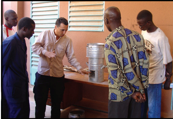
Artisans learn about a Rocket stove at the Burkina Faso stove workshop
