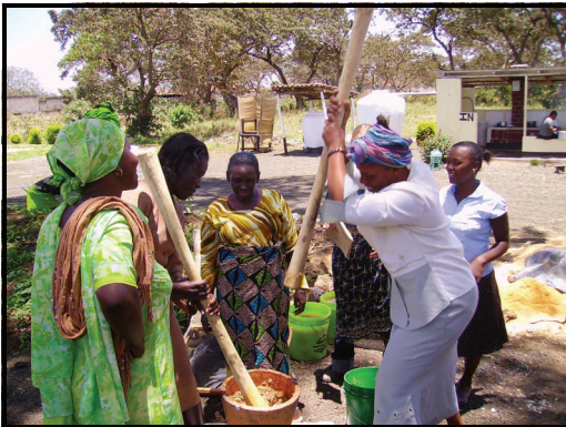
WODSTA group members pulping raw materials to be used for sawdust briquettes
