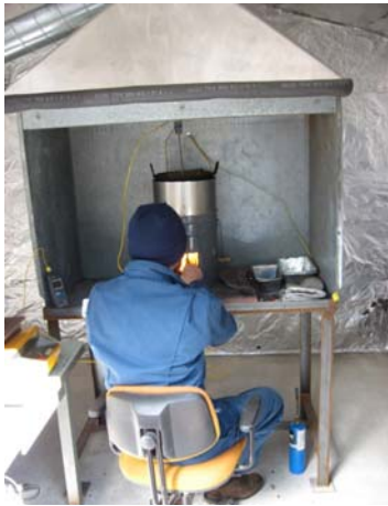
Stove testing in emissions hood
