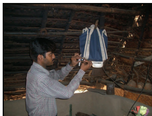
Indoor air pollution sampling equipment including a UCB Particle Monitor
