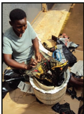
Mrs. Mariam makes a hay basket, arranging different layers of grass, plastic, newspaper, cotton, sponge and old newspaper inside the basket.
