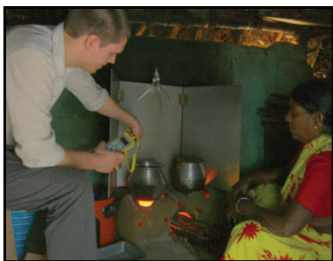
Berkeley Air staff monitoring emissions from a 2-pot traditional mud stove in Tamil Nadu, India
