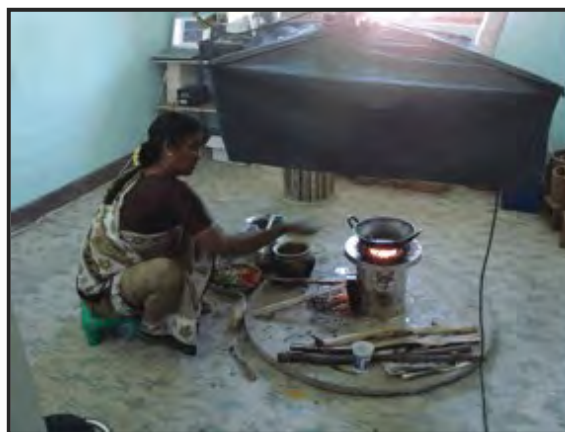
Conducting testing on wood stoves under an emissions hood
