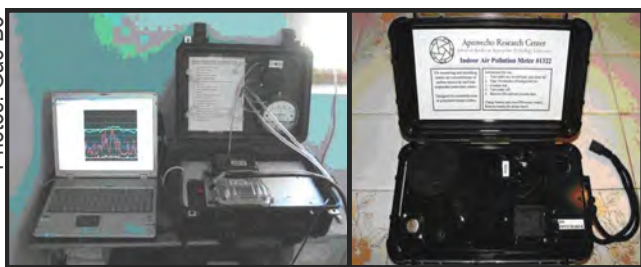
Equipment at the PEMS Control Panel and Indoor Air Pollution Meter at the CAU Testing Center for Household Biomass Stoves
