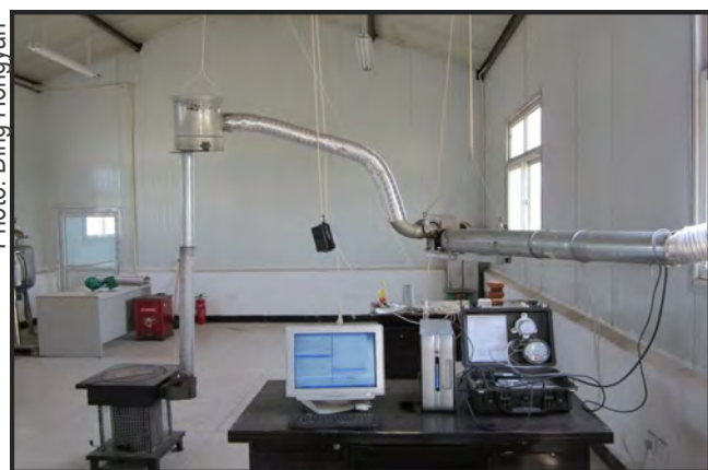
Stove Performance Monitoring System
