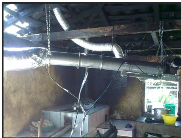
PEMS installed in a rural household to evaluate emissions during real use.
