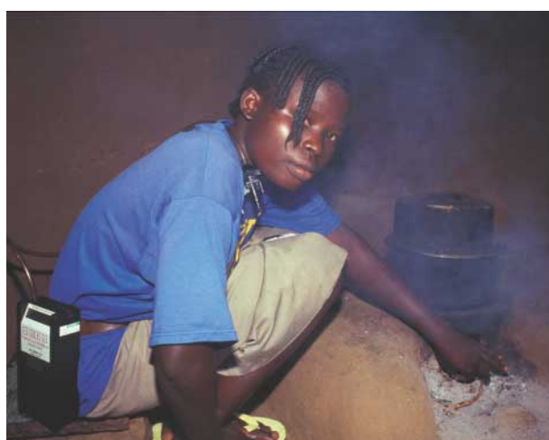
Monitoring personal exposure using the pump and filter method
