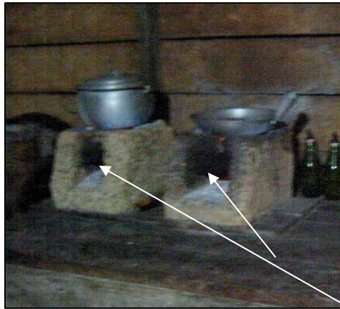
Fig 3. Cement Stove I
