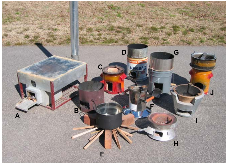
Figure 1 – Stoves tested: A. Ecostove, B. VITA, C. UCODEA charcoal, D. WFP rocket, E. 3-stone fire, F. Philips, G. 6-brick rocket, H. Lakech charcoal, I. NLS, J. UCODEA rocket
